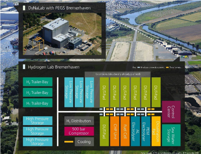
Figure 1: Overview of the test facilities in Bremerhaven with the HLB layout (bottom) and the DyNaLab with PEGS
