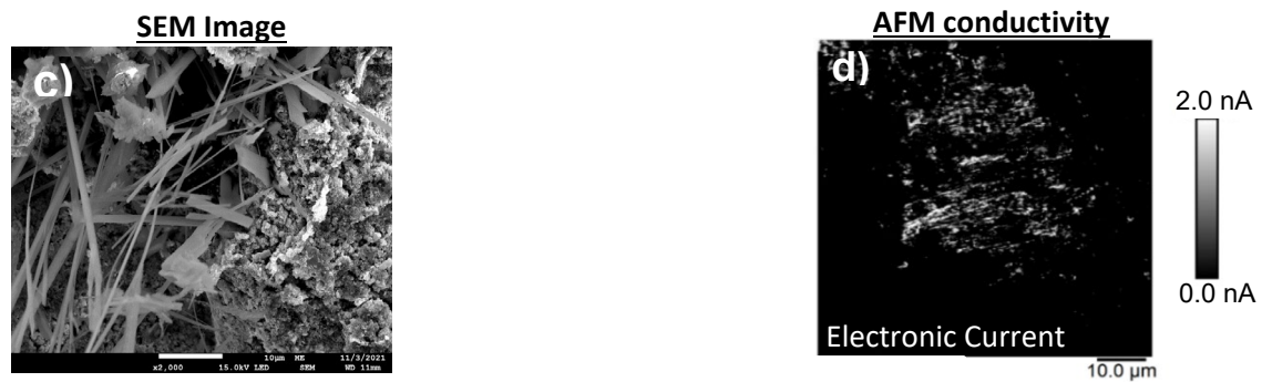
Figure 1: a) Performance comparison between initial performance and after operation. Images of the physical analysis b) AFM topography of the anodic BPP, c) SEM of the anode-side CCM, d) AFM conductivity measurement of the anodic BPP
